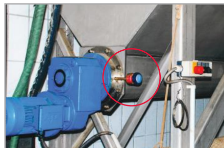
Sludge thickening process: Lubrication of bearing at screw press
