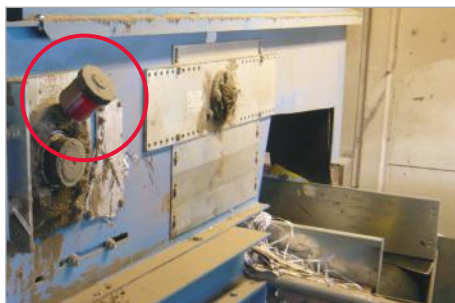
Lubrication of flange bearing on a conveyor
