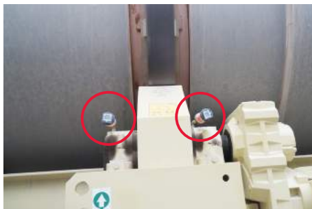
Lubrication of thrust roller bearings on a drum dryer
