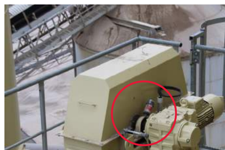
Roller bearing lubrication on a filler elevator
