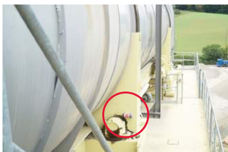
Lubrication of thrust roller bearings on a parallel drum
