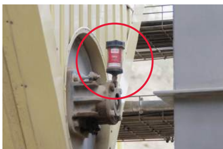
Flange bearing lubrication on a trough screw conveyor (dedusting)
