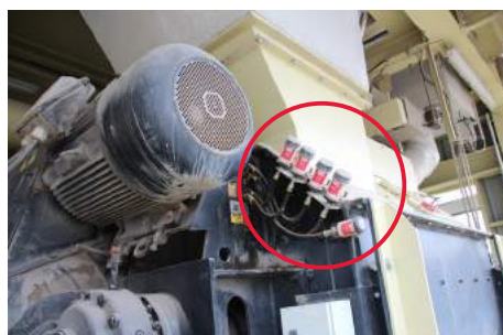
Lubrication of mixing shafts and mixer flaps
