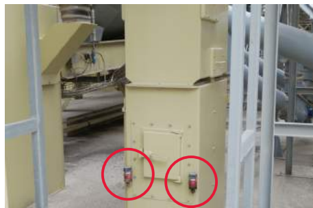
Footstep bearing lubrication on a filler
