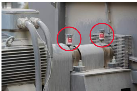
Pillow block lubrication on an exhauster
