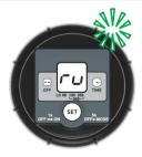
If the short run cycle is successful the lubricator will return to normal operation, showing the time setting.
