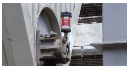
Flange bearing lubrication on a trough screw conveyor (dedusting)
