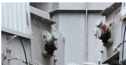
Roller bearing lubrication on conveyors
